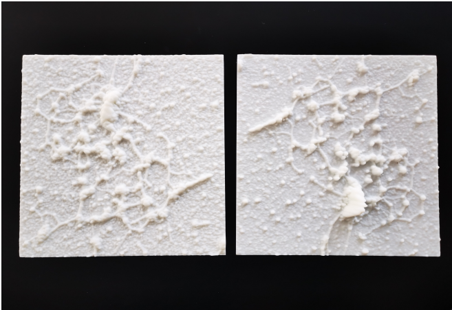
Figure 3: Experiments of manufacturing, first prototype of Sample1, wet vegetal matter under decomposition (soil #1). 3d printing, opaque white resin. On the left, we used a logarithmic vertical scale, and on the right, a linear vertical scale.
